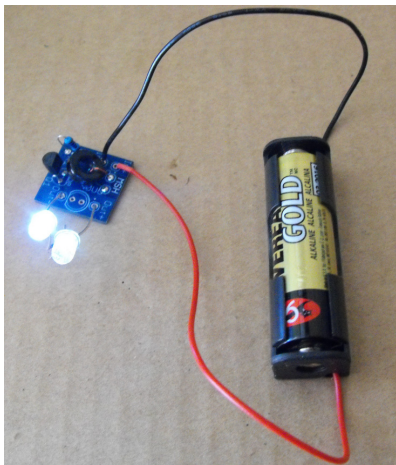
Running two white LEDs in series.
